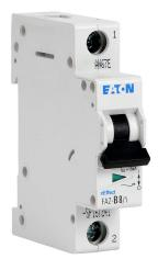
Eaton miniature supplementary protector, 8A, 277 VAC / 48 VDC, 1-pole, B curve, thermal magnetic, 10kA @ 277 VAC interrupting rating, 35mm DIN rail mount.
