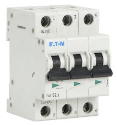
Eaton miniature supplementary protector, 7A, 480Y / 277 VAC / 96 VDC, 3-pole, B curve, thermal magnetic, 10kA @ 480Y/277 VAC interrupting rating, 35mm DIN rail mount.
