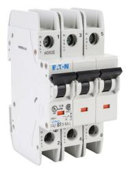
Eaton miniature circuit breaker, current-limiting, 7A, 240 VAC / 96 VDC, 3-pole, B curve, thermal magnetic, 10kA @ 240 VAC interrupting rating, 35mm DIN rail mount.
