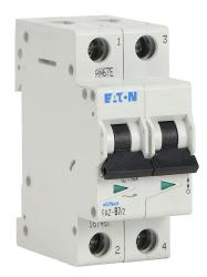
Eaton miniature supplementary protector, 7A, 480Y / 277 VAC / 96 VDC, 2-pole, B curve, thermal magnetic, 10kA @ 480Y/277 VAC interrupting rating, 35mm DIN rail mount.
