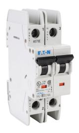
Eaton miniature circuit breaker, current-limiting, 7A, 480Y / 277 VAC / 96 VDC, 2-pole, B curve, thermal magnetic, 10kA @ 480Y/277 VAC interrupting rating, 35mm DIN rail mount.
