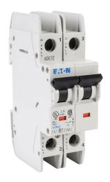
Eaton miniature circuit breaker, current-limiting, 7A, 240 VAC / 96 VDC, 2-pole, B curve, thermal magnetic, 10kA @ 240 VAC interrupting rating, 35mm DIN rail mount.
