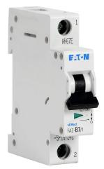
Eaton miniature supplementary protector, 7A, 277 VAC / 48 VDC, 1-pole, B curve, thermal magnetic, 10kA @ 277 VAC interrupting rating, 35mm DIN rail mount.
