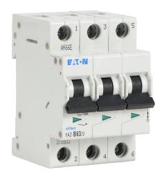
Eaton miniature supplementary protector, 63A, 480Y / 277 VAC / 96 VDC, 3-pole, B curve, thermal magnetic, 5kA @ 480Y/277 VAC interrupting rating, 35mm DIN rail mount.
