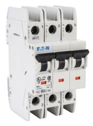
Eaton miniature circuit breaker, current-limiting, 63A, 240 VAC / 96 VDC, 3-pole, B curve, thermal magnetic, 10kA @ 240 VAC interrupting rating, 35mm DIN rail mount.
