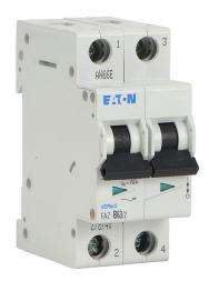
Eaton miniature supplementary protector, 63A, 480Y / 277 VAC / 96 VDC, 2-pole, B curve, thermal magnetic, 5kA @ 480Y/277 VAC interrupting rating, 35mm DIN rail mount.
