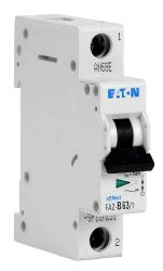
Eaton miniature supplementary protector, 63A, 277 VAC / 48 VDC, 1-pole, B curve, thermal magnetic, 5kA @ 277 VAC interrupting rating, 35mm DIN rail mount.
