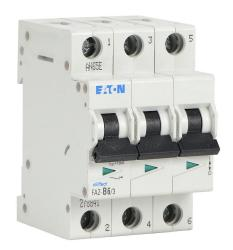
Eaton miniature supplementary protector, 6A, 480Y / 277 VAC / 96 VDC, 3-pole, B curve, thermal magnetic, 10kA @ 480Y/277 VAC interrupting rating, 35mm DIN rail mount.
