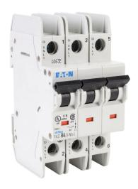
Eaton miniature circuit breaker, current-limiting, 6A, 240 VAC / 96 VDC, 3-pole, B curve, thermal magnetic, 10kA @ 240 VAC interrupting rating, 35mm DIN rail mount.
