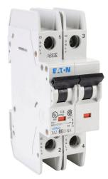
Eaton miniature circuit breaker, current-limiting, 6A, 480Y / 277 VAC / 96 VDC, 2-pole, B curve, thermal magnetic, 10kA @ 480Y/277 VAC interrupting rating, 35mm DIN rail mount.
