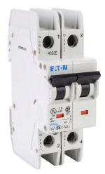
Eaton miniature circuit breaker, current-limiting, 6A, 240 VAC / 96 VDC, 2-pole, B curve, thermal magnetic, 10kA @ 240 VAC interrupting rating, 35mm DIN rail mount.
