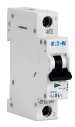
Eaton miniature supplementary protector, 6A, 277 VAC / 48 VDC, 1-pole, B curve, thermal magnetic, 10kA @ 277 VAC interrupting rating, 35mm DIN rail mount.
