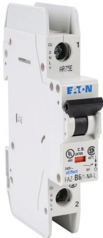
Eaton miniature circuit breaker, current-limiting, 6A, 240 VAC / 48 VDC, 1-pole, B curve, thermal magnetic, 10kA @ 240 VAC interrupting rating, 35mm DIN rail mount.
