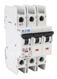
Eaton miniature circuit breaker, current-limiting, 50A, 240 VAC / 96 VDC, 3-pole, B curve, thermal magnetic, 10kA @ 240 VAC interrupting rating, 35mm DIN rail mount.
