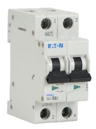
Eaton miniature supplementary protector, 50A, 480Y / 277 VAC / 96 VDC, 2-pole, B curve, thermal magnetic, 5kA @ 480Y/277 VAC interrupting rating, 35mm DIN rail mount.
