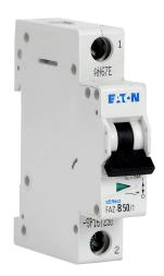
Eaton miniature supplementary protector, 50A, 277 VAC / 48 VDC, 1-pole, B curve, thermal magnetic, 5kA @ 277 VAC interrupting rating, 35mm DIN rail mount.
