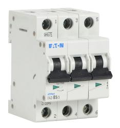
Eaton miniature supplementary protector, 5A, 480Y / 277 VAC / 96 VDC, 3-pole, B curve, thermal magnetic, 10kA @ 480Y/277 VAC interrupting rating, 35mm DIN rail mount.
