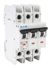
Eaton miniature circuit breaker, current-limiting, 5A, 480Y / 277 VAC / 96 VDC, 3-pole, B curve, thermal magnetic, 10kA @ 480Y/277 VAC interrupting rating, 35mm DIN rail mount.
