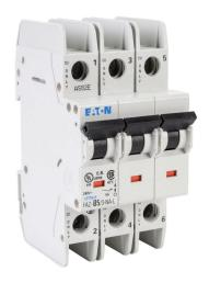
Eaton miniature circuit breaker, current-limiting, 5A, 240 VAC / 96 VDC, 3-pole, B curve, thermal magnetic, 10kA @ 240 VAC interrupting rating, 35mm DIN rail mount.
