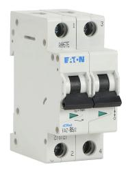
Eaton miniature supplementary protector, 5A, 480Y / 277 VAC / 96 VDC, 2-pole, B curve, thermal magnetic, 10kA @ 480Y/277 VAC interrupting rating, 35mm DIN rail mount.
