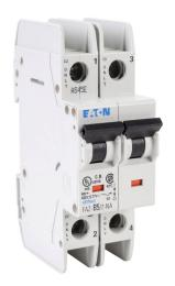
Eaton miniature circuit breaker, current-limiting, 5A, 480Y / 277 VAC / 96 VDC, 2-pole, B curve, thermal magnetic, 10kA @ 480Y/277 VAC interrupting rating, 35mm DIN rail mount.
