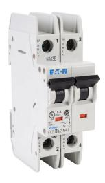
Eaton miniature circuit breaker, current-limiting, 5A, 240 VAC / 96 VDC, 2-pole, B curve, thermal magnetic, 10kA @ 240 VAC interrupting rating, 35mm DIN rail mount.
