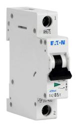
Eaton miniature supplementary protector, 5A, 277 VAC / 48 VDC, 1-pole, B curve, thermal magnetic, 10kA @ 277 VAC interrupting rating, 35mm DIN rail mount.
