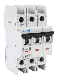
Eaton miniature circuit breaker, current-limiting, 40A, 240 VAC / 96 VDC, 3-pole, B curve, thermal magnetic, 10kA @ 240 VAC interrupting rating, 35mm DIN rail mount.
