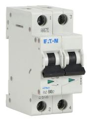
Eaton miniature supplementary protector, 40A, 480Y / 277 VAC / 96 VDC, 2-pole, B curve, thermal magnetic, 5kA @ 480Y/277 VAC interrupting rating, 35mm DIN rail mount.
