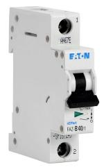
Eaton miniature supplementary protector, 40A, 277 VAC / 48 VDC, 1-pole, B curve, thermal magnetic, 5kA @ 277 VAC interrupting rating, 35mm DIN rail mount.
