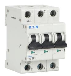
Eaton miniature supplementary protector, 4A, 480Y / 277 VAC / 96 VDC, 3-pole, B curve, thermal magnetic, 10kA @ 480Y/277 VAC interrupting rating, 35mm DIN rail mount.
