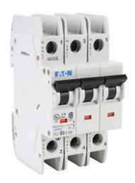
Eaton miniature circuit breaker, current-limiting, 4A, 480Y / 277 VAC / 96 VDC, 3-pole, B curve, thermal magnetic, 10kA @ 480Y/277 VAC interrupting rating, 35mm DIN rail mount.
