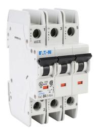
Eaton miniature circuit breaker, current-limiting, 4A, 240 VAC / 96 VDC, 3-pole, B curve, thermal magnetic, 10kA @ 240 VAC interrupting rating, 35mm DIN rail mount.
