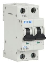
Eaton miniature supplementary protector, 4A, 480Y / 277 VAC / 96 VDC, 2-pole, B curve, thermal magnetic, 10kA @ 480Y/277 VAC interrupting rating, 35mm DIN rail mount.
