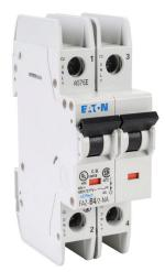
Eaton miniature circuit breaker, current-limiting, 4A, 480Y / 277 VAC / 96 VDC, 2-pole, B curve, thermal magnetic, 10kA @ 480Y/277 VAC interrupting rating, 35mm DIN rail mount.
