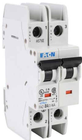
Eaton miniature circuit breaker, current-limiting, 4A, 480Y / 277 VAC / 96 VDC, 2-pole, B curve, thermal magnetic, 10kA @ 480Y/277 VAC interrupting rating, 35mm DIN rail mount.
