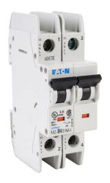
Eaton miniature circuit breaker, current-limiting, 4A, 240 VAC / 96 VDC, 2-pole, B curve, thermal magnetic, 10kA @ 240 VAC interrupting rating, 35mm DIN rail mount.
