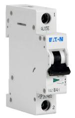
Eaton miniature supplementary protector, 4A, 277 VAC / 48 VDC, 1-pole, B curve, thermal magnetic, 10kA @ 277 VAC interrupting rating, 35mm DIN rail mount.
