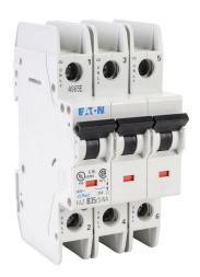
Eaton miniature circuit breaker, current-limiting, 35A, 240 VAC / 96 VDC, 3-pole, B curve, thermal magnetic, 10kA @ 240 VAC interrupting rating, 35mm DIN rail mount.
