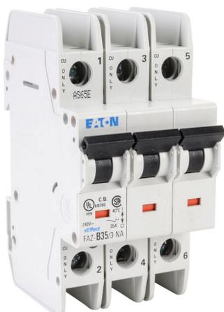
Eaton miniature circuit breaker, current-limiting, 35A, 240 VAC / 96 VDC, 3-pole, B curve, thermal magnetic, 10kA @ 240 VAC interrupting rating, 35mm DIN rail mount.
