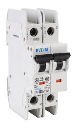
Eaton miniature circuit breaker, current-limiting, 35A, 240 VAC / 96 VDC, 2-pole, B curve, thermal magnetic, 10kA @ 240 VAC interrupting rating, 35mm DIN rail mount.
