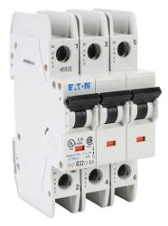
Eaton miniature circuit breaker, current-limiting, 32A, 480Y / 277 VAC / 96 VDC, 3-pole, B curve, thermal magnetic, 10kA @ 480Y/277 VAC interrupting rating, 35mm DIN rail mount.
