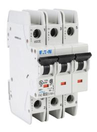
Eaton miniature circuit breaker, current-limiting, 32A, 240 VAC / 96 VDC, 3-pole, B curve, thermal magnetic, 10kA @ 240 VAC interrupting rating, 35mm DIN rail mount.
