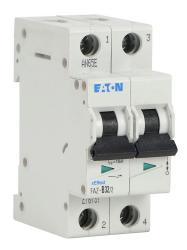
Eaton miniature supplementary protector, 32A, 480Y / 277 VAC / 96 VDC, 2-pole, B curve, thermal magnetic, 10kA @ 480Y/277 VAC interrupting rating, 35mm DIN rail mount.
