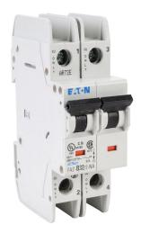
Eaton miniature circuit breaker, current-limiting, 32A, 480Y / 277 VAC / 96 VDC, 2-pole, B curve, thermal magnetic, 10kA @ 480Y/277 VAC interrupting rating, 35mm DIN rail mount.
