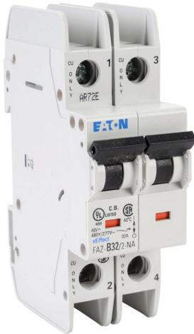
Eaton miniature circuit breaker, current-limiting, 32A, 480Y / 277 VAC / 96 VDC, 2-pole, B curve, thermal magnetic, 10kA @ 480Y/277 VAC interrupting rating, 35mm DIN rail mount.
