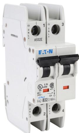
Eaton miniature circuit breaker, current-limiting, 32A, 240 VAC / 96 VDC, 2-pole, B curve, thermal magnetic, 10kA @ 240 VAC interrupting rating, 35mm DIN rail mount.
