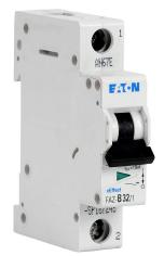
Eaton miniature supplementary protector, 32A, 277 VAC / 48 VDC, 1-pole, B curve, thermal magnetic, 10kA @ 277 VAC interrupting rating, 35mm DIN rail mount.
