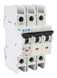
Eaton miniature circuit breaker, current-limiting, 30A, 480Y / 277 VAC / 96 VDC, 3-pole, B curve, thermal magnetic, 10kA @ 480Y/277 VAC interrupting rating, 35mm DIN rail mount.
