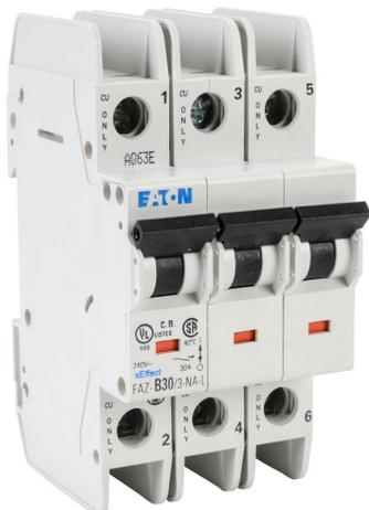
Eaton miniature circuit breaker, current-limiting, 30A, 240 VAC / 96 VDC, 3-pole, B curve, thermal magnetic, 10kA @ 240 VAC interrupting rating, 35mm DIN rail mount.
