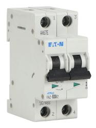
Eaton miniature supplementary protector, 30A, 480Y / 277 VAC / 96 VDC, 2-pole, B curve, thermal magnetic, 10kA @ 480Y/277 VAC interrupting rating, 35mm DIN rail mount.
