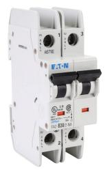
Eaton miniature circuit breaker, current-limiting, 30A, 480Y / 277 VAC / 96 VDC, 2-pole, B curve, thermal magnetic, 10kA @ 480Y/277 VAC interrupting rating, 35mm DIN rail mount.
