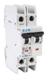
Eaton miniature circuit breaker, current-limiting, 30A, 240 VAC / 96 VDC, 2-pole, B curve, thermal magnetic, 10kA @ 240 VAC interrupting rating, 35mm DIN rail mount.
